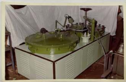
VACUUM IMP. SYSTEM FOR TRANSFORMER COILS.
