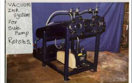
VACUUM IMP. SYSTEM FOR TRANSFORMER COILS FOR ELECTRONICS INDUSTRY.
