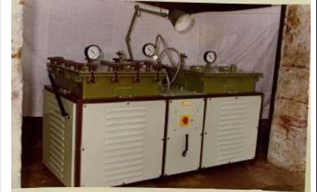
VACUUM IMP. SYSTEM FOR SUB. PUMP ROTORS.
